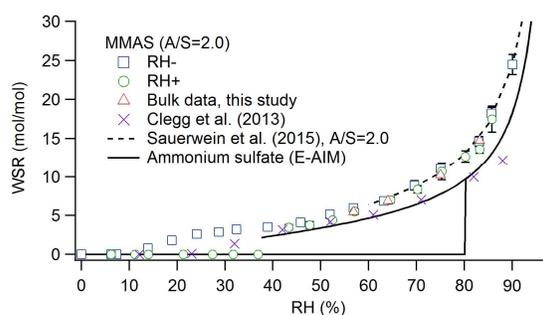
Figure 1. Hygroscopicity of MMAS (A/S=2.0) and comparison with literature data. RH+ and RH- indicate data points obtained during humidification and dehumidification in the RH cycle, respectively.
