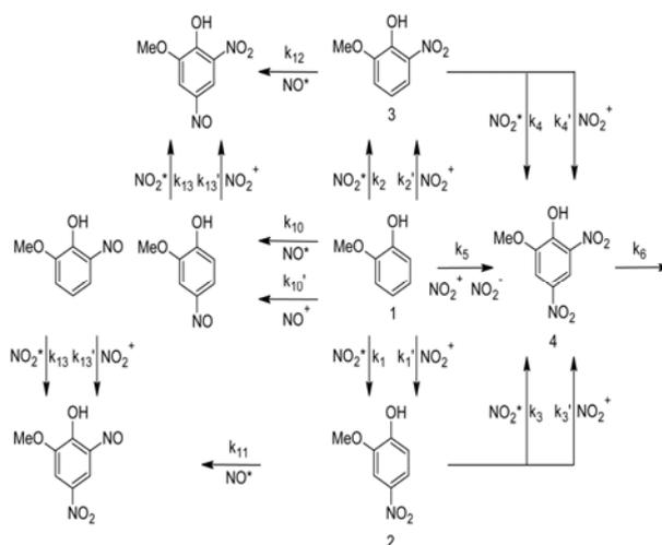
Figure 1. Proposed reaction mechanism of guaiacol nitration in acidic aqueous solution. 1 guaiacol (GUA), 2 4-nitroguaiacol (4NG), 3 6-nitroguaiacol (6NG), and 4 4,6-dinitroguaiacol (DNG). The model does not distinguish between 4- and 6-nitrosoguaiacol (NOG).
