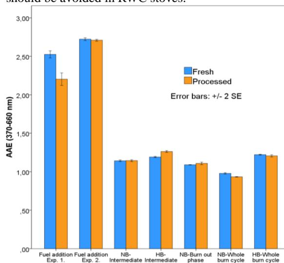
Figure 1. AAE for different burn phases and comparison of fresh vs. photochemical processed aerosol.
