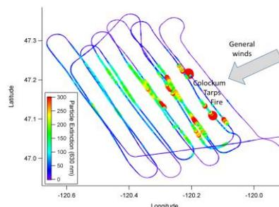
Figure 1. Particulate extinction measured downwind of the Colockum Tarps fire 30 July 2013.
