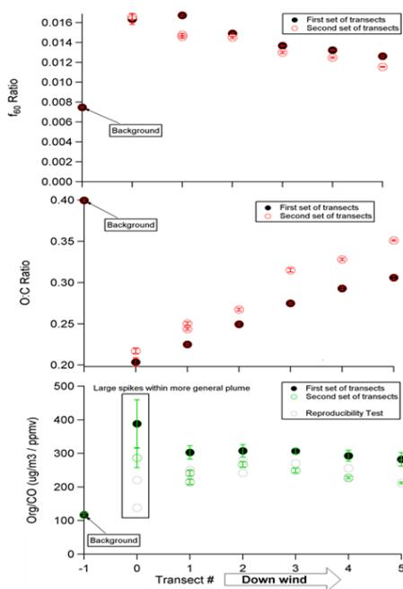
Figure 2. Particulate organic mass and chemical composition measured downwind.
