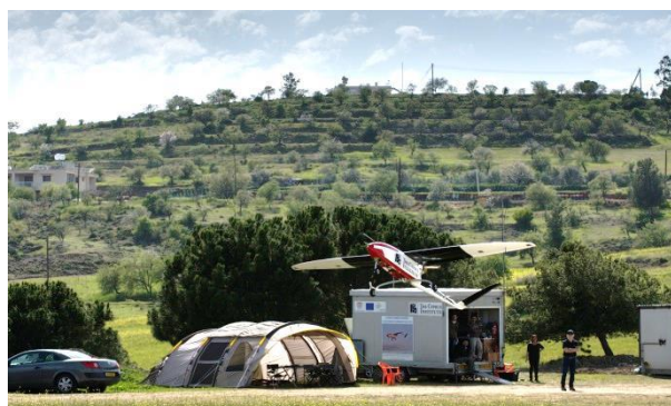
Figure 3: Take-off of one the CyI UAV dedicated to gas/aerosol observations at the Agia Marina Xyliatou airfield.
