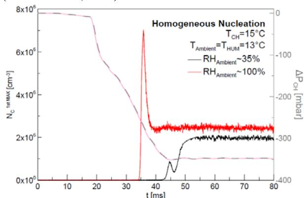
**Figure 1.** Pressure drop (magenta) and scattered light signals (red and black) at two different RH conditions.
