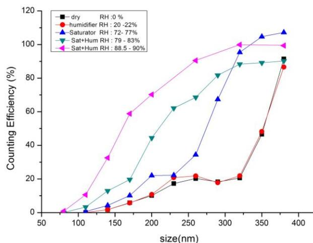
Figure 2. FMI-ACIT's counting efficiency for different particle sizes at 5 ranges of relative humidity ( $Q = 2.1\text{lpm}$ )
