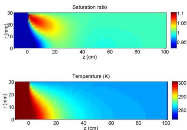
Figure 1. Calculated Saturation ratio and temperature profiles inside the flow tube condenser (flow direction from left to right) ( $T_{\text{sat.}} = 299.3\text{K}$   $T_{\text{preh.}} = 300.6\text{K}$   $T_{\text{cond.}} = 280.8\text{K}$ ,  $Q = 2.1\text{lpm}$ )
