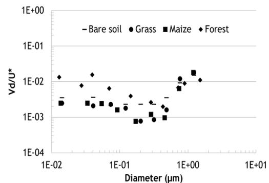
Figure 1: Dry deposition velocity dimensionless with the friction velocity for bare soil, grass, maize and forest.
