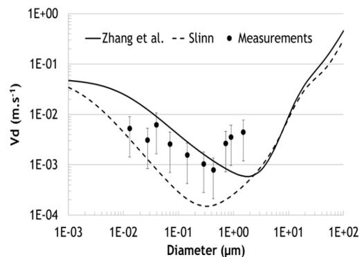
Figure 2: Comparison between measurements and two models on the forest.
