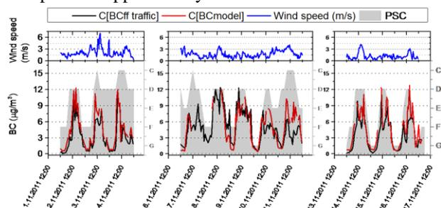
Figure 1: Measured and modeled parameters: BC apportioned to traffic with the Aethalometer model (C[BCff traffic]); BC calculated with EMISENS and diffusion model (C[BCmodel]); Pasquill stability classes (PSC); and Maribor airport wind speed.
