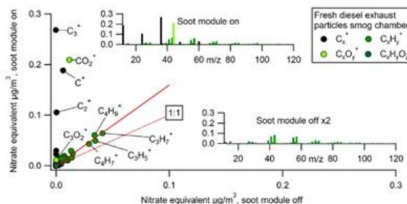
Figure 1: Mass spectra of fresh diesel exhaust particles. Scatterplot data recorded with soot module on versus off. Hydrocarbon ion intensities increase uniformly. Carbon clusters and carbon and oxygen containing ions increase by highly variable factors, indicating refractory components.
