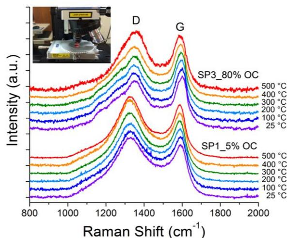
Figure 1. Raman spectra of soot samples with different OC content during oxidation. Insert: photo of setup for *in situ* RM measurements.
