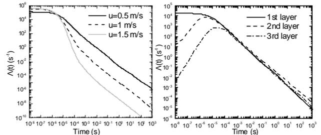
Figure 1: Effect of exposure time and friction velocity on  $\Lambda(t)$  of the top layer of a two-layer deposit of 70  $\mu\text{m}$  stainless steel particles (left).  $\Lambda(t)$  for a three-layer deposit of the same particles at friction 0.3 m/s (right).
