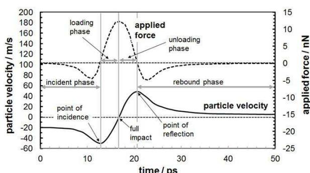
Fig.1. MD simulation of the temporal evolution of particle velocity and applied force for the different phases of a particle-wall collision: incident phase (approach), contact phase (loading/unloading) and rebound phase.
