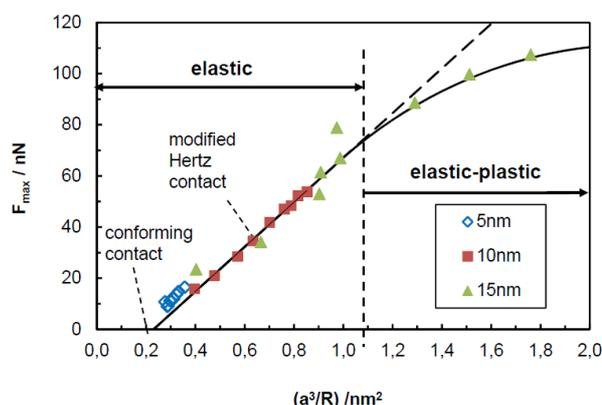
Fig.2. Maximum force vs. Hertz parameter for Ag nanoparticles impacting on a mica target
