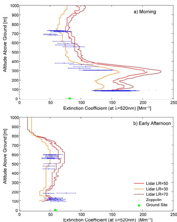
Figure 1. Comparison between in-situ (ground based and airborne) and remote sensing (Lidar) measurements.
