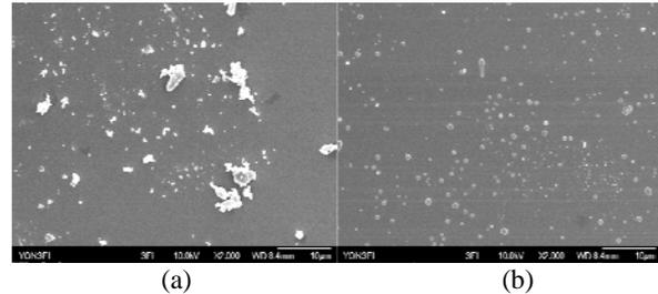
Fig. 1 SEM pictures of Minor (a) and Major (b) outlets for the cutoff diameter of 1  $\mu\text{m}$  (Magnification =  $\times 2,000$ ).
