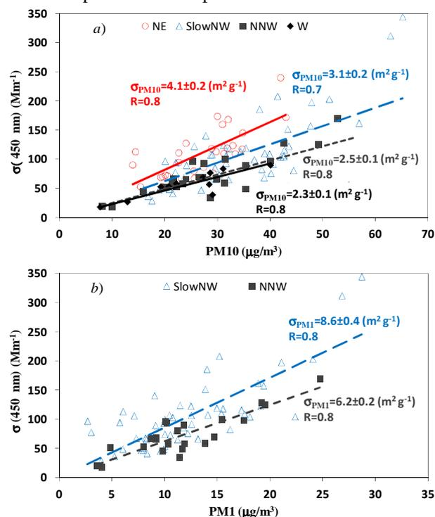
Figure 1. Scattering coefficient versus a) PM10 and b) PM1 mass concentrations.
