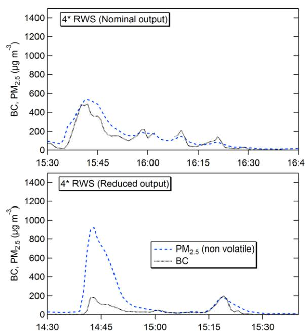
Figure 1. Time evolution of BC and PM<sub>2.5</sub> (non volatile) concentrations using the 4\* RWS at nominal and reduced outputs.
