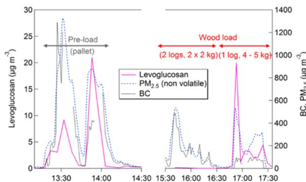
Figure 2. Time evolution of levoglucosan, BC and PM<sub>2.5</sub> (non volatile) concentrations using the 4\* RWS for different combustion conditions and wood loads (nominal output, wood load: beech, 12% moisture).
